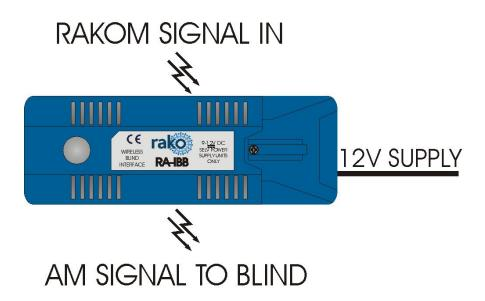
The RA-IBB comes with a 12V supply fitted with a 13A plug.
