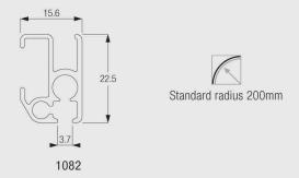
Due to the enclosed channels, this curtain track can be forward and reverse bent. The standard bending radius of 200mm can be reduced to as low as 100mm for reverse and forward bends if no overlap arm is used.
