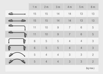
Straight tracks can be extended beyond 6m by using a connecting bridge and intermediate pulley.
