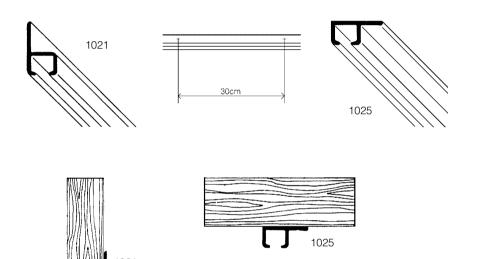
If future access to track ends for either 1021 or 1025 is difficult or impossible, then the profile can be slotted at one end using the 7030 slotting tool. This allows for easy removal or addition of extra gliders if so required at a later date. The slot is stopped using the 3032 spring endstop.
