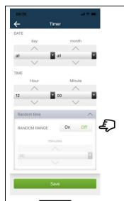
Time for Action can be randomised, this feature can be left off or turned on by press here.
