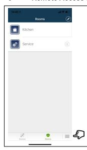
To SETUP Remote Access and Voice Control first press the three horizontal lines. 6.1
