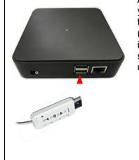
After programming all your products onto the transmitter stick (see separate instructions) plug the stick into the server unit.
