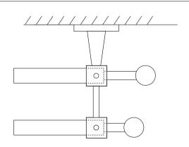
All 19mm poles should be fitted so that the pole ends within the bracket. The grub screw tightens up on the pole causing it to grip the finial.
