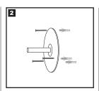
Attach the back plates to the wall using the screws provided.
