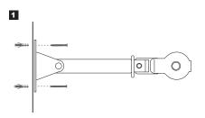
Measure and secure the tension cord pulley in place using the screws provided.
