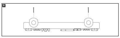
Attach the securing screws through the bracket locking the pole in position.
